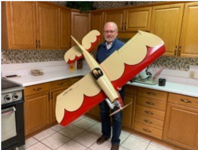
This is a Great Planes kit with an O.S. Max 46AX II turning a 11 X 7 prop. Multiplex Cockpit SX 9 transmitter and Futaba S3151 servos. True to its name, it can fly slow!
